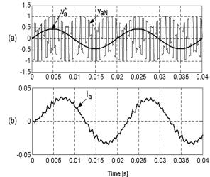
Fig: 4. Direct method: Venturini, typical waveforms. (a) Output voltage  $v_{aN}$  (b) output current  $i_a$
