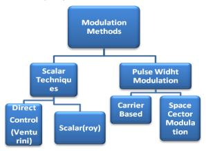
Fig: 2. Block Diagram of Modulation Techniques
