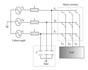
Fig: 1. Block diag. of MC
